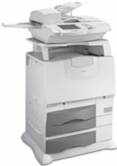
FIGURE 5-6. Multifunction printer has four functions: color printer, scanner, plain-paper fax, and copier. (Courtesy of Lexmark International.)
